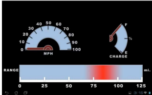
Figure 3: Display of estimated range of electric car, with uncertainty [12].
