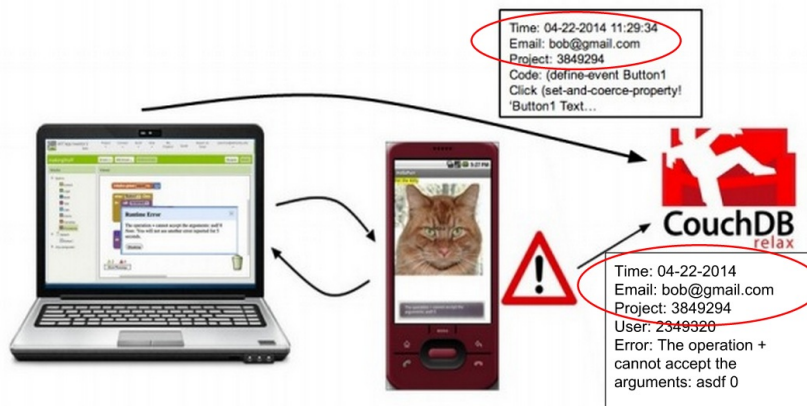
Figure 7-1: When an error is generated, reports are sent from both the Blocks Editor and the device.
