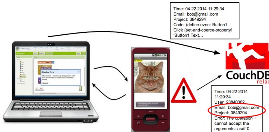
Figure 1-11: When an error is generated, reports are sent from both the Blocks Editor and the device.
