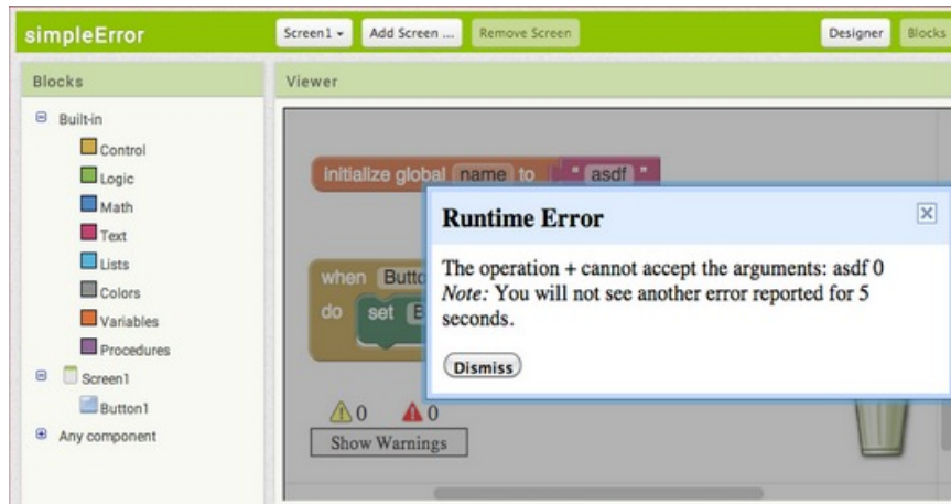
Figure 1-5: A runtime error generated by an app displayed in the Blocks Editor
