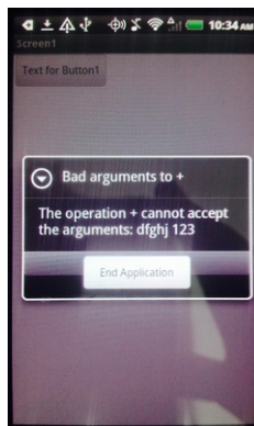
Figure 5-1: In App Inventor Classic, a running app generates an error and a message appears on the screen of the device.
