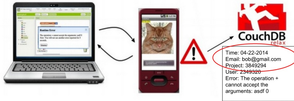
Figure 1-10: An error generated on the device while the user is in live development mode is sent to a database on the cloud
