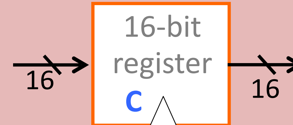
Registers (local data storage)
