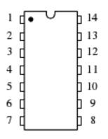
**Bottom left** pin is almost always connected to ground (0V)
