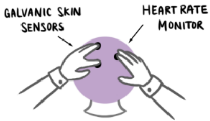
Figure 3. The left hand is placed on two galvanic skin sensors, and the right hand is placed on a pulse sensor.
