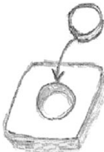
Fig. 1 The physical properties of the constraint affords placement of the token in the indentation
