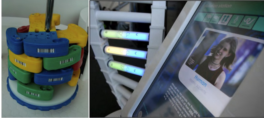
Fig. 4.9 The Inside DNA exhibition at the Glasgow Science Centre. Left: visitors create a DNA strand by stacking colored blocks with barcodes onto a shaft, and the strand is then read by rotating the tower past a reader. Right: at another exhibit, rotating the lighted tubes selects DNA. An attached screen then explains which kind of animal has been created (images courtesy: Glasgow Science Centre, 2009).
