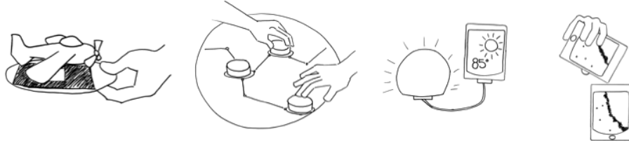
Fig. 3.1 Research areas related to TUIs. From left to right: Tangible Augmented Reality, virtual objects (e.g., airplane) are “attached” to physically manipulated objects (e.g., card); Tangible Tabletop Interaction, physical objects are manipulated upon a multi-touch surface; Ambient Displays, physical objects are used as ambient displays; Embodied User Interfaces, physical devices are integrated with their digital content.
