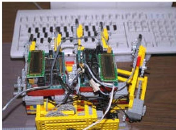
**Fig. 10.** In the *Handroid* project, a student used two Handy Boards to control a six-motor LEGO hand that could (slowly) type any specified string of characters. The *Handroid* moved back and forth along a gear rack, and reflectance sensors at the tips of each of its fingers counted keys as it moved.
