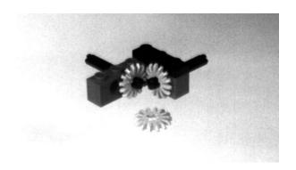
The bevel gears are used to change the angle of rotation of shafts in a gear train with a 1:1 ratio. In this case, they are used to effect a change in the horizontal plane.
