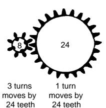
When the 8-tooth gear rotates 3 times, it advances the meshed gear by a total of 24 teeth. Since the meshed gear has 24 teeth, it rotates exactly once. Hence this configuration produces a 3:1 ratio of gear reduction: three turns of the input gear causes one turn of the output gear.
