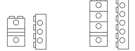
Figure 2: Creating Vertical Spacings with Two-Unit and Four-Unit Horizontal Measures
