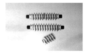
This diagram shows an arrangement of worm gears. At the bottom is the basic worm gear, two horizontal LEGO units in length. At the top is an unsuccessful attempt to put two worm gears on the same shaft. In the middle is the successful attempt. When placing multiple worm gears on a shaft, the trick is to try all four possible orientations to find the one that works.
