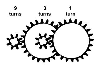
Figure 5: 9-to-1 Gear Reduction with Ganging
