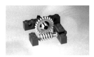
Figure 7: Using the Worm Gear
