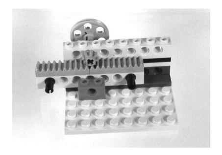
The gear driving the gear rack is often referred to as the "pinion," as in "rack-and-pinion steering," which uses the transverse motion of the gear rack to orient wheels. The 8—tooth gear is a good candidate to drive the rack because of the gear reduction it achieves—one revolution of the gear moves the rack by eight teeth.
