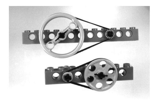
There are three sizes of pulley wheel: the tiny one, which doubles as a stop bush, the medium-sized one, which doubles as a tire hub, and the large-sized one, which is sometimes used as a steering wheel in official LEGO plans.
