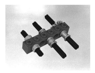
The standard 1-LEGO-long stop bush (upper axle, front) is not the only part that can act as a bushing (axle holder). Use the small pulley wheel (middle axle) to act as a half-sized spacer—it also grabs tighter than the full bush. In a pinch, the bevel gear (upper axle, back) makes a great bushing. Finally, the nut-and-bolt parts (lower axle) can be used to make a tight connection (if you can find them).
