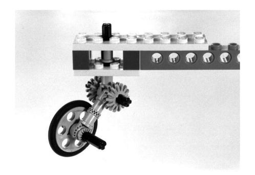
Several clichés are used to construct this caster wheel. The vertical axle is trapped between two plates, but allowed to rotate, using the trick shown in Figure 24. The angled joint down to the wheel is done using toggle joints in the configuration suggested in Figure 26, and the final mounting of the wheel is done using the toggle joint per Figure 27.
