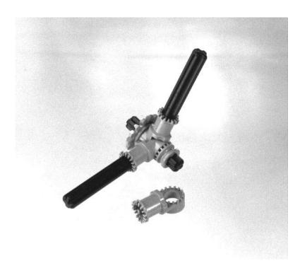
Figure 26: Two Toggle Joints
