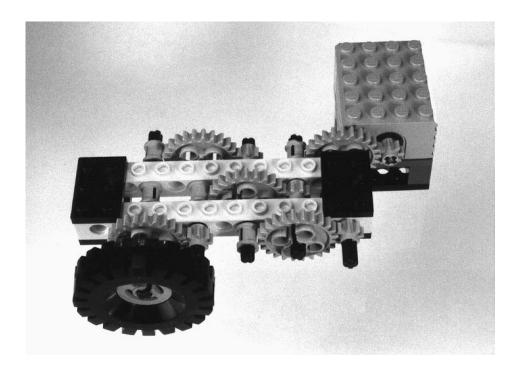
A five-stage reduction using 8– and 24–tooth gears creates a 243-to-1 reduction in this sample LEGO geartrain. Note the need for three parallel planes of motion to prevent the gears from interfering with one another. Four 2×3 LEGO plates are used to hold the beams square and keep the axles from binding.
