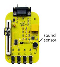
The sound sensor value block is similar to Scratch's loudness block: both blocks measure how loud sounds are.
