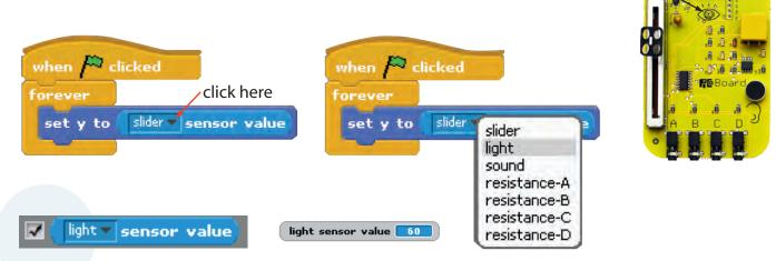
Select "light" and check the box to make a new sensor watcher appear on the stage. The readings on this watcher indicate the brightness of the light reaching the **light sensor** on the PicoBoard.
