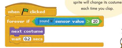
You can use sensor values to control araphic effects. Watch the cat whirl when you blow into the sound sensor.
