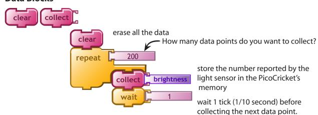
**collect** stores a data point (a number from 0 to 100) in the PicoCricket's memory. A PicoCricket can collect up to 200 data points. Click on **graph** to see a graph of the collected data.
