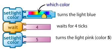
Sets the LED's color and turns it on. You can set the color by using the color slider, or choosing a number between 0 and 100. Colors are numbered as follows:
