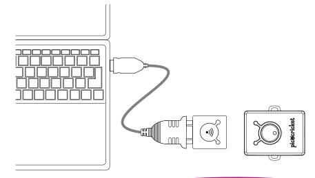
The PicoCricket Kit includes a USB-serial cable for connecting the Beamer to a USB port on your computer. Alternatively, you can connect the Beamer to a serial port, using a standard serial cable (not included).
