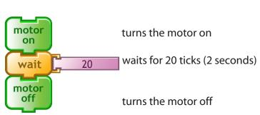
**motoroff** makes the motor coast to a stop. If you want the motor to stop more abruptly or more gently, try using the **brake** and **coast** commands in the <u>PicoBlocks Text Language</u>.
