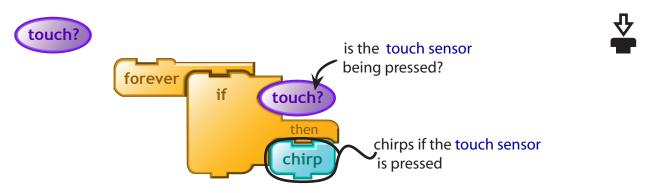
**touch?** reports true when the touch sensor is being pressed. The example above will make the PicoCricket chirp continuously while you are pressing the button on the touch sensor. If you want to chirp only once each time you push the button, you should make a stack similar to the one shown below:
