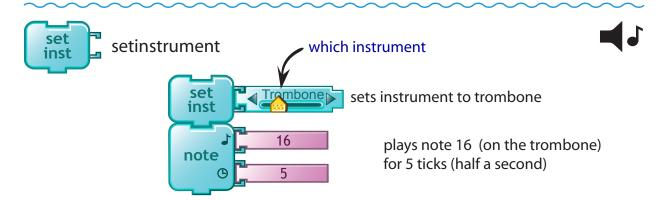
Sets the instrument to be used for subsequent notes or melodies. You can select the instrument with the slider or attach a number between 0 and 100. **setinstrument 0** sets the note or melody with the PicoCricket's beeper.
