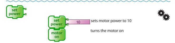
**setpower** takes values between 0 (no power) and 100 (strongest power). **setpower** does not turn on the motor, it only sets the power.
