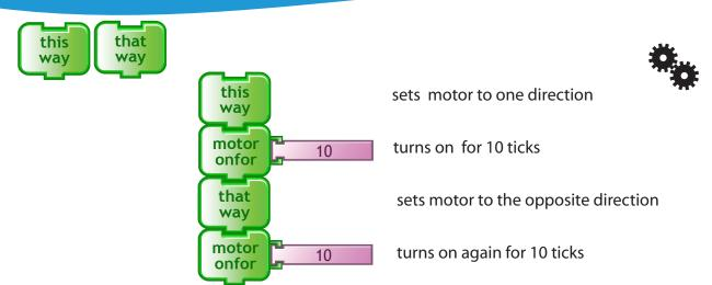
**thisway** sets the motor in one direction, **thatway** sets it in the other direction. Which direction is which depends on how the motor is plugged in. **thisway** and **thatway** do not turn on the motor, they only set the direction.
