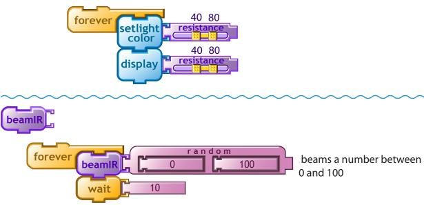
**beamIR** beams a number to another PicoCricket via infrared (IR). To use this command, you need two PicoCrickets: one beaming the IR signal, the other receiving the IR signal. See example for **IR** block below. We recommend using numbers in the range 0 to 100. Numbers outside this range may produce unexpected results.
