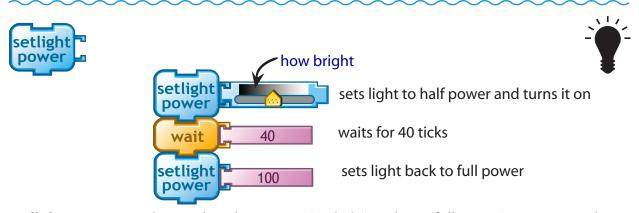
**setlightpower** can take numbers between 0 (no light) and 100 (full power). You can set the power by using the slider or a number block.
