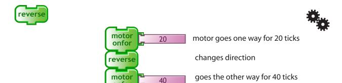
**reverse** causes the motor to change the direction in which it is spinning. **reverse** does not turn the motor on, it only changes the direction.
