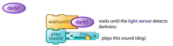
dark? reports true if the light sensor detects the brighness to be less than 15.
