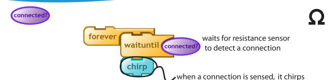
connected? reports true if the resistance sensor detects a resistance of less than 50.
