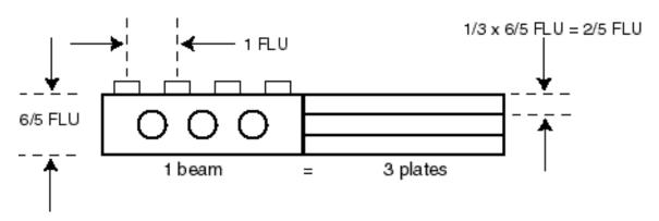
Three plates have the same vertical dimension as a beam (6/5 FLU), so each plate has a thickness of  $1/3 \times 6/5 = 2/5 \text{ FLU}$ . Plates can be used to adjust the vertical spacing so that it is an integral number of FLUs. For example, the beams in the stack below have holes separated by exactly 2 FLU in the vertical direction:
