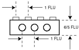
One key to strong LEGO structures is **vertical bracing**, using **beams** and **pegs.** Try stacking a bunch of beams together and vertically bracing them. Chances are the holes don't line up. Why?
