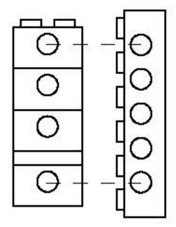
In the above stack, each beam is equivalent to three plates, and there are effectively three beams and one plate in the stack, so
