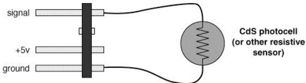
The light sensors we use are made using a **photocell**, which is made a substance whose electrical resistance decreases when it is illuminated with visible light. As you've probably noticed, in Handy Logo the sensor values get smaller as the intensity of light increases. (We'll explain why next week.) *Sciborg* has a pair of light sensors in front, which can serve as eyes. (With a relatively
