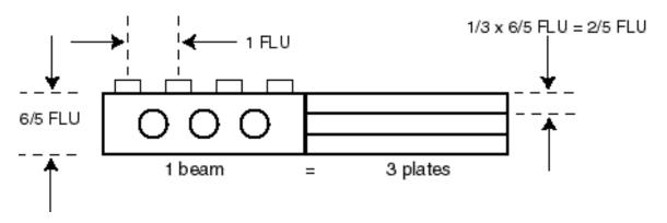
Three plates have the same vertical dimension as a beam (6/5 FLU), so each plate has a thickness of  $1/3 \times 6/5 = 2/5$  FLU. Plates can be used to adjust the vertical spacing so that it is an integral number of FLUs. For example, the beams in the stack below have holes separated by exactly 2 FLU in the vertical direction:
