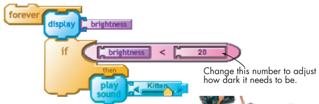
Cast a shadow on the brightness sensor
