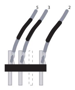
Step 2 - Connect the cable to the breadboard
