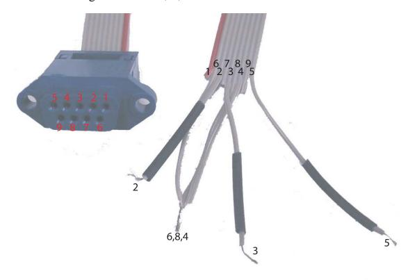
Now solder wires number 2, 3, and 5 to a male header (obtained from Digi-Key part number S1032-36-ND), as shown in the figure below. After the soldering is complete, slip the heat—shrinkable tubing over the solder joint and heat with a heat gun to shrink the tubing and insulate the joint.
