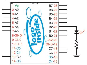
Suppose a red LED is connected to pin B2 of the LogoChip as shown above. Here is what the Logo code that would make the LED flash once might look like:
