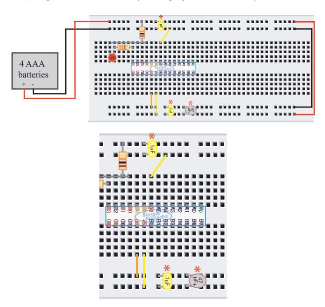
The purpose of adding these "bypass capacitors" is to "keep the busses quiet"; that is to try to help the battery maintain a constant voltage difference between
