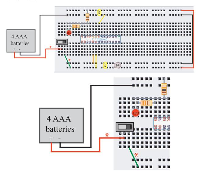
The negative terminal from the battery pack should remain connected directly to the ground bus while the positive terminal from the battery pack should be connected to the middle pin of the slide switch. When the slide switch is in the left-position there should be no connection between the positive terminal of the battery pack and the power bus on the breadboard. Flipping the slide switch to the right-position should make this connection.
