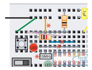
When the LogoChip is turned on it checks to see if the resonator is present, and if it is it automatically makes the necessary adjustments to run at the higher rate. you can check this by running the benchmark test:
