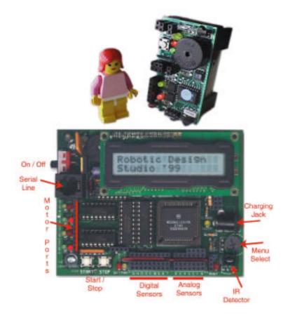
**Fig. 1.** Programmable bricks. The top device is a Cricket, which is about the size of a 9 volt battery. The bottom device is a Handy Board, a palm-sized robotic computer. The devices and LEGO figure are shown at roughly the same scale.
