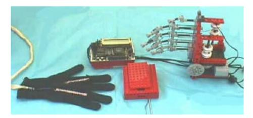
**Fig. 9.** *Paper, Scissors, Rock* is a robotic version of the common children's game. A robotic hand with four moveable fingers and a stationary thumb is capable of closing itself into a fist for rock, throwing out just two fingers for scissors or throwing out four fingers for paper. The robot randomly "decides" what to throw. The human opponent wears a glove equipped with bend sensors so that the robot "knows" what the human threw and can determine the winner.
