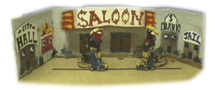
**Fig 5.** *Western Duel* starred a pair of robotic gunslingers performing the classic pace, turn and fire sequence found in countless cowboy movies. It featured a sense of drama.(the winner was determined randomly) and brilliant mechanical design (the loser slouched over).
