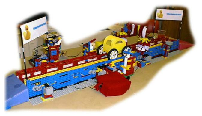
**Fig. 6.** Inspired by a visit to a local auto wash, the 6 foot long *Rubber Ducky's Car Wash* featured soap bubbles generated by fans blowing on a bubble wands, gentle mists of water supplied by LEGO driven aerosol cans, and a visually spectacular buffing action provided by colorful felt brushes.
