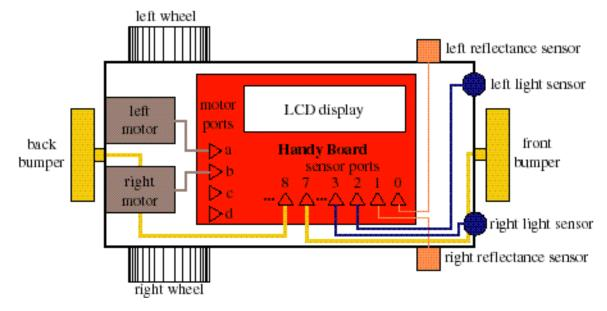
**Fig. 2.** Schematic of *SciBorg* (top view). It has two motors (connected to motor ports a and b); two reflectance sensors (connected to sensor ports 0 and 1); two light sensors (connected to sensor ports 2 and 3); and two bumpers (connected to sensor ports 7 and 8).
