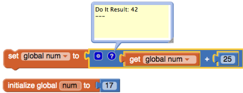
Figure 10. Invoking DoIt on an expression block displays the value of that block, as calculated by the interpreter on the device.
