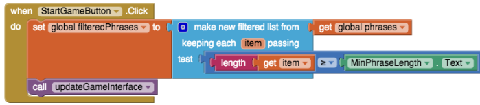
Fig. 2. The Click handler with our new filter block (labeled make new filtered list from ). It declares a baked-in item parameter that ranges over all input list items and is referenced from the test expression.
