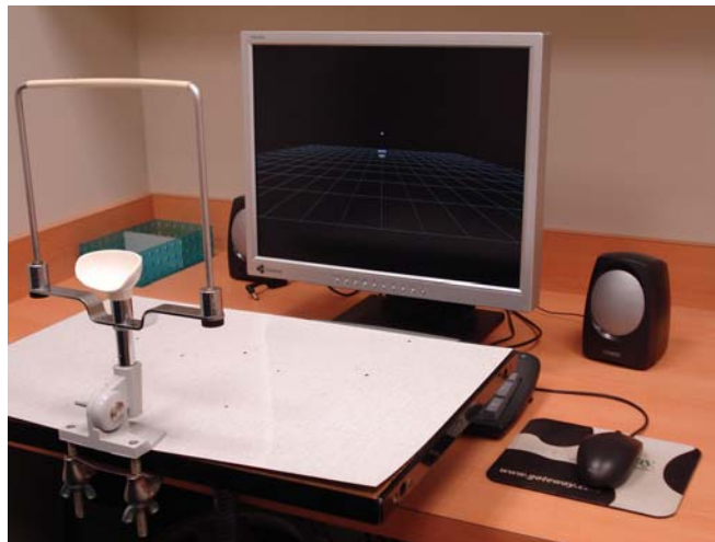
Figure 5. Experimental setup showing the display screen with the catching task simulation, chin rest and computer mouse. Actual experimental sessions were conducted in a dark room.
