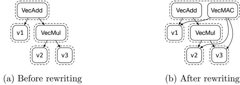
Figure 2.4: An E-graph before and after applying a rewrite rule for fused multiply-accumulate. Solid boxes are nodes and represent program terms. Dashed boxes represent equivalence classes. After rewriting, the `VecAdd` and `VecMAC` terms are in the same equivalence class.
