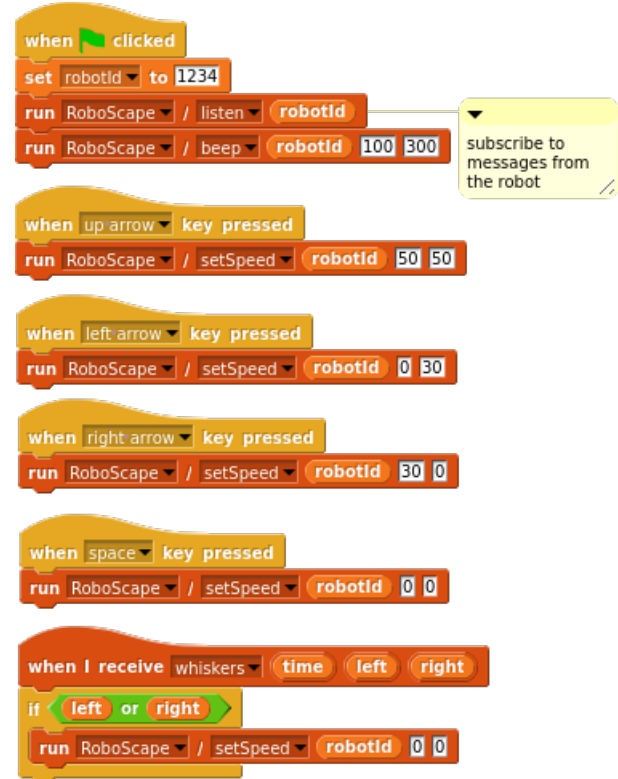
Figure 4. A partial RoboScape project implementing driving the robot with keyboard commands
