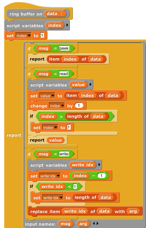
Figure 1: Creating an anonymous dispatch procedure that serves as a circular buffer object
