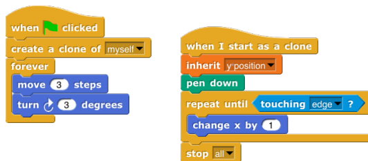
Figure 2: Using a clone and inheritance of the parent's y-position to draw a sine-curve
