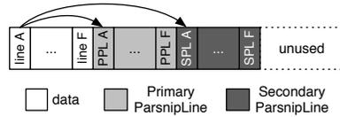
Figure 2: Parsnip's physical address space layout.
