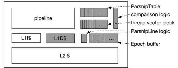
Figure 6: Parsnip additions (shaded) to a conventional core.
