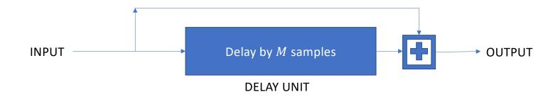
In the basic delay setup, an input signal is added to a copy of the same signal that has been passed through a delay unit which delays the incoming signal by some unit of time. For now, we will deal with *audible* delays, meaning ones where we can perceive the two signals as separate but simultaneous streams of sound. When the delay between signals gets incredibly small other interesting effects can occur.
