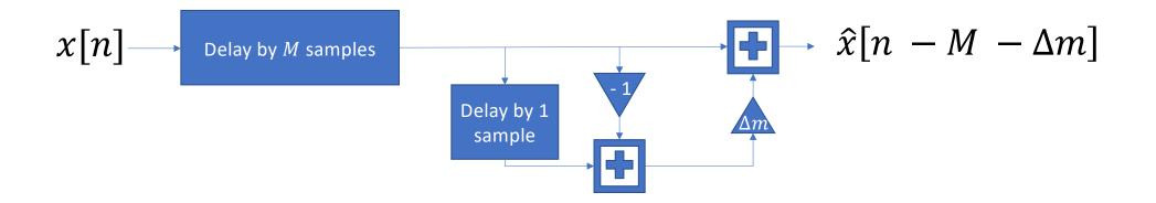
A block diagram of the linearly interpolated delay. The triangles are equivalent to multiplication.
