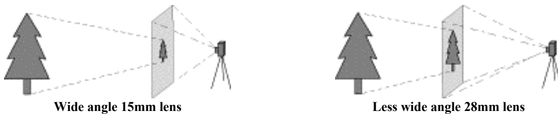
Wider angle lenses make objects appear smaller in the image but provide a greater vertical field of view
