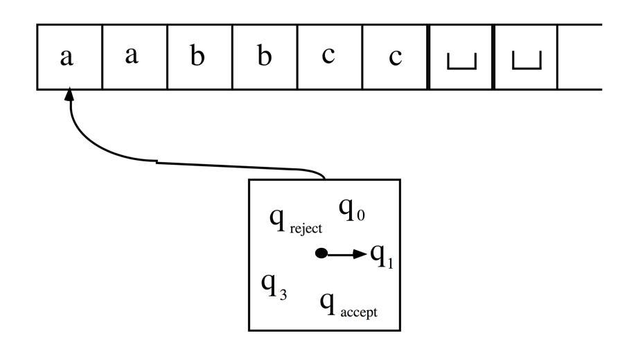
**Definition.** A *Turing Machine* is a 7-tuple,  $M = (Q, \Sigma, \Gamma, \delta, q_0, q_{accept}, q_{reject}), Q, \Sigma, \Gamma$  are finite sets,
