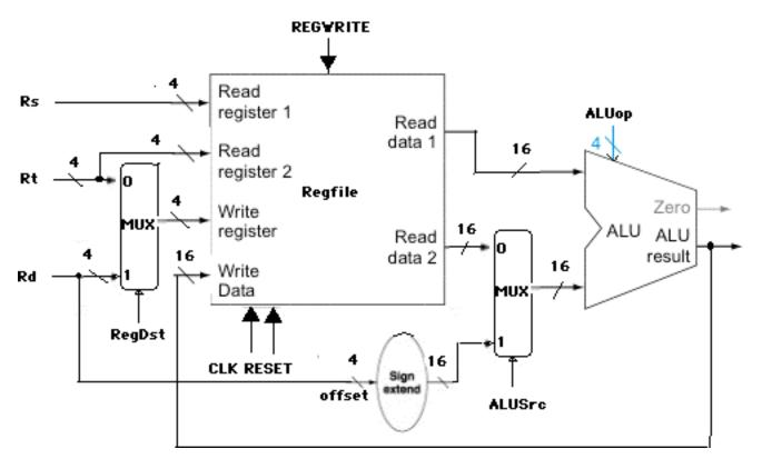
Display Read data 1 and Read data 2 from the Regfile, and the ALU result using hex displays.
