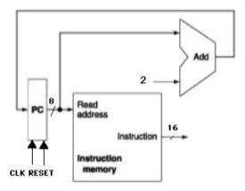
Add an 8-bit register (**Reg-8** in LogicWorks) and an 8-bit adder to your Instruction Memory circuit from last week (you can find this in *parts.cct* from the Google group).
