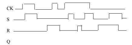
4. Assume you have a clocked SR flip-flop, that is activated on the positive edge of the clock. Draw Q given the same CK, S, and R:
