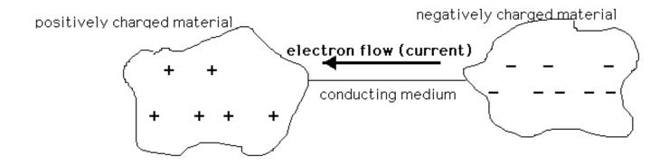
Rate at which electrons flow through = current(A).
