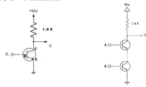
**AND** – uses 3 transistors (send the output of a NAND through another transistor acting as a NOT gate to complement the result):
