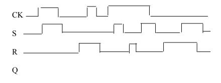
5. Assume you have a clocked SR **flip-flop**, that is activated on the positive edge of the clock. Draw Q given the same CK, S, and R:
