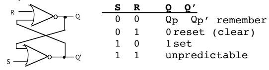
What does **unpredictable** mean? Notice in a NOR gate, if either input = 1 to a gate, its output = 0 (1 is a deterministic input):
