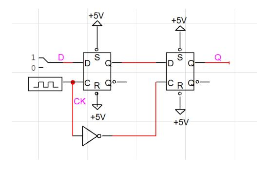
So, the input D will not be passed from the first latch to the second latch until the clock goes low.
