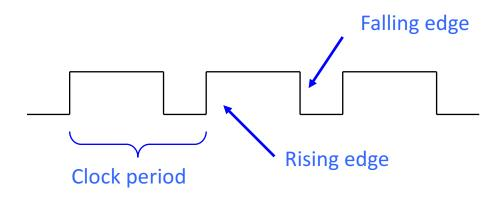
A clock controls when to update a sequential logic element's state.
