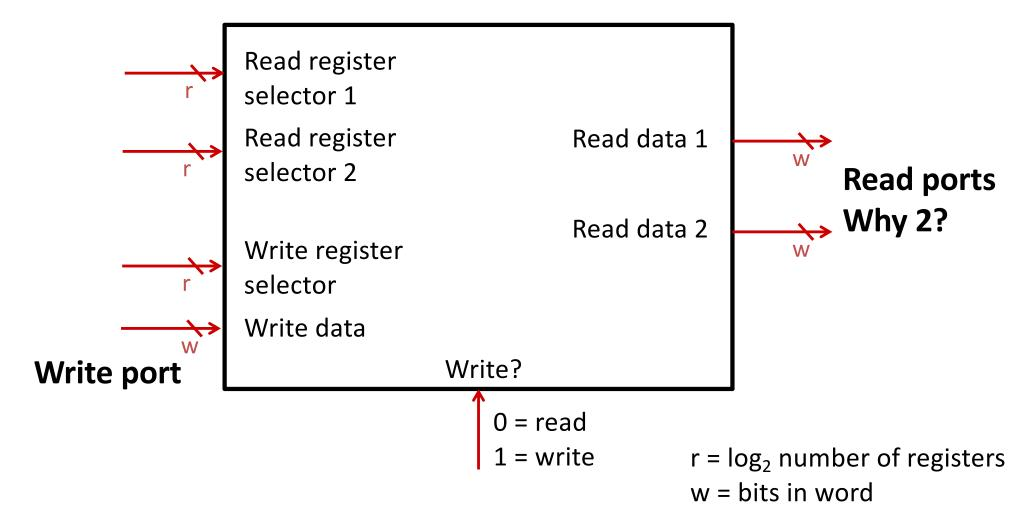
Array of registers, with register selectors, write/read control, input port for writing data, output ports for reading data.
