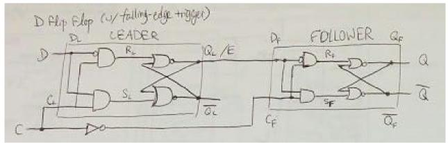
b. Simulate the behavior of the flip-flop you drew, given the waveforms of D and C:
