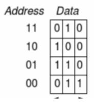
In addition to the flip-flops, and although it is not shown in the diagram above, a memory also contains multiplexer and decoder circuits to select which value is being accessed. For example, a 256x16 RAM contain 256 16-bit values.
