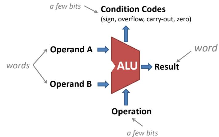
Hardware unit for arithmetic and bitwise operations.
