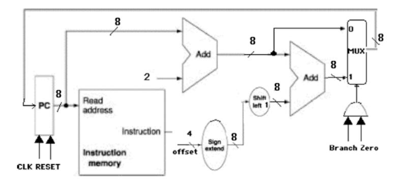
A MUX (multiplexer) selects the next value of the PC, either PC+2 (calculated by the first adder), or PC + 2 + 2\*offset (calculated by the second adder).
