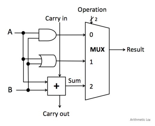
The **Operation** (a 2-bit value), selects which operation should be produced as the **Result**:
