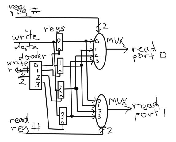
Although a register file contains multiple registers, it is still a fairly small memory, and is a special purpose circuit for the CPU.
