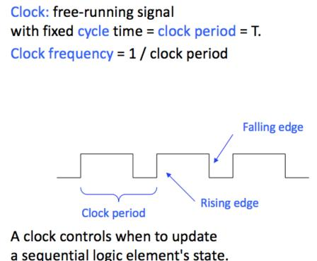
In a clocked latch, whenever the clock is high, the outputs/state of the latch can change.
