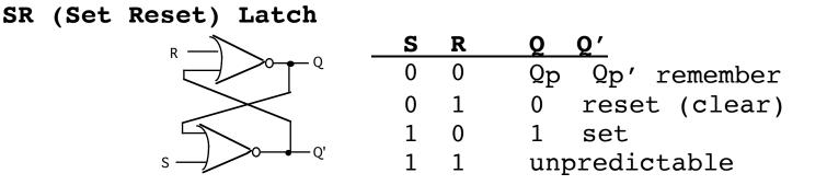
What does **unpredictable** mean? Notice in a NOR gate, if either input = 1 to a gate, its output = 0 (1 is a deterministic input):
