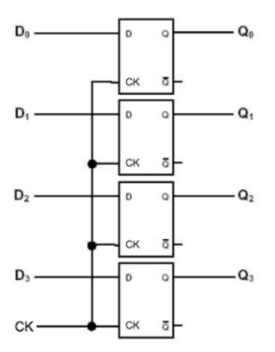
Registers are used to represent single n-bit value in a Computer Processing Unit (CPU).
