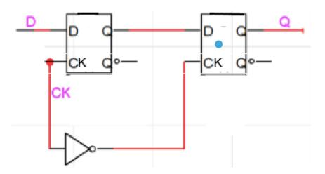
So, the input D will not be passed from the first latch to the second latch until the clock goes low.
