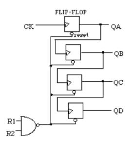
The output of the first T flip-flop, QA, serves as the clock to QB. So, QB only changes when QA falls from 1 to 0 (on the negative edge). QB therefore only changes half as frequently as QA.
