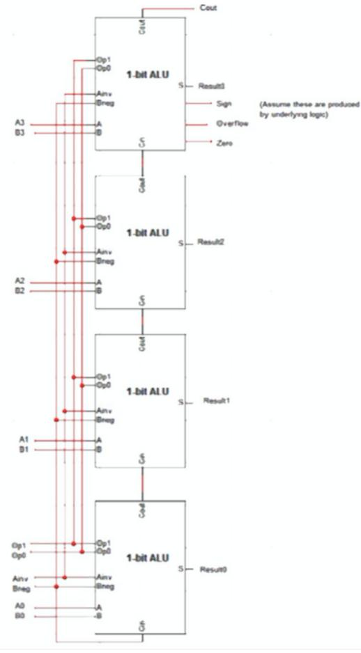
How do you produce the Sign, Overflow, and Zero bits?
