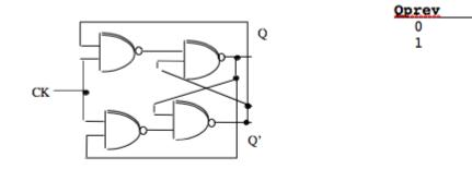
The T flip-flop can be abstracted to the following device (the **reset** input allows you to initialize the device to a value of 0):
