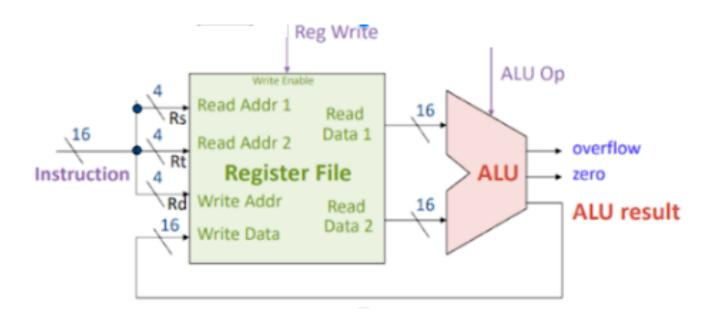
This circuit can execute the arithmetic and logical operations including **ADD,SUB,AND**, and **OR**. The general form is:
