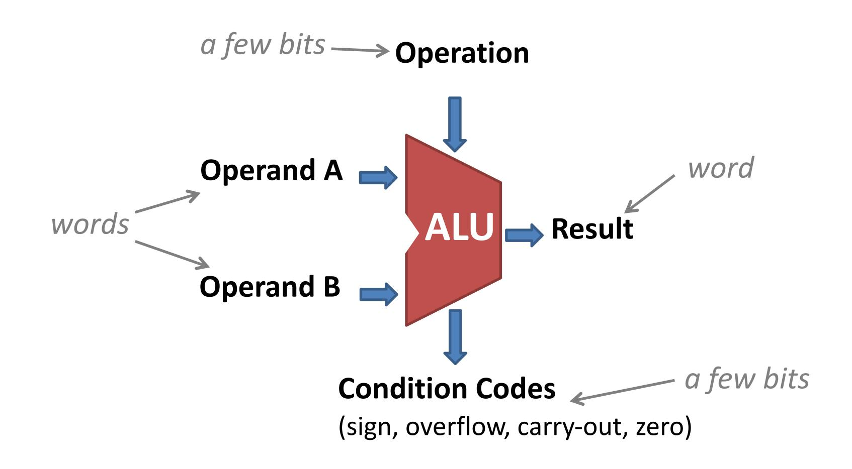
Hardware unit for arithmetic and bitwise operations.
