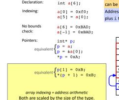
Arrays are adjacent memory locations storing the same type of data. a is a name for the array's base address, can be used as an immutable pointer. Address of a[i] is base address a plus i times element size in bytes.
