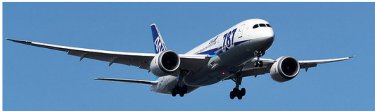
"... a **Model 787 airplane** ... can lose all alternating current (AC) electrical power ... caused by a **software counter** internal to the GCUs that will **overflow** after **248 days** of continuous power. We are issuing this AD to prevent loss of all AC electrical power, which could result in **loss of control of the airplane.**"
