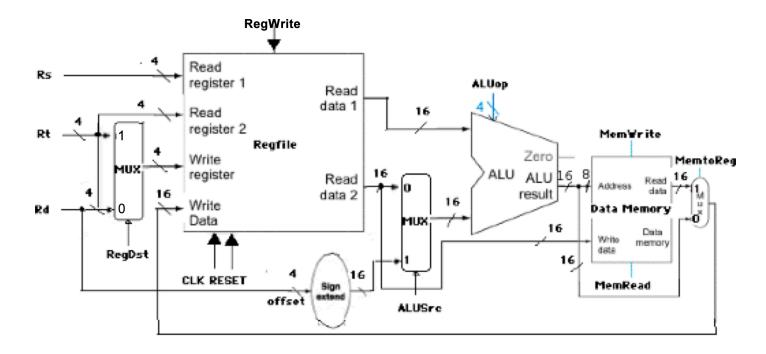
The control lines for the various multiplexers and Data Memory can be produced as a simple function of the opcode, as defined in the following table:
