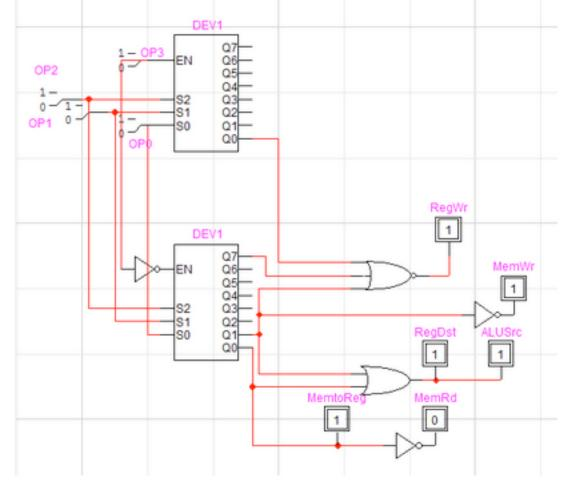
Write a function for each control line, or use a decoder to produce the signals. Paste your design here:
