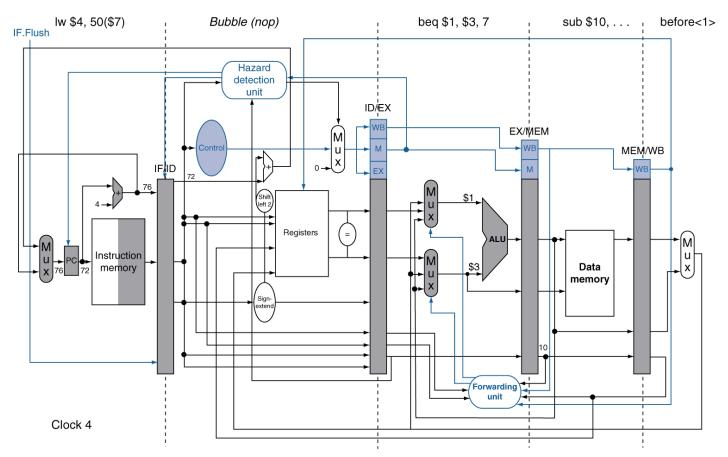
9. The following diagram in the text and in lecture explains the modifications needed in the pipeline to handle hazards:
