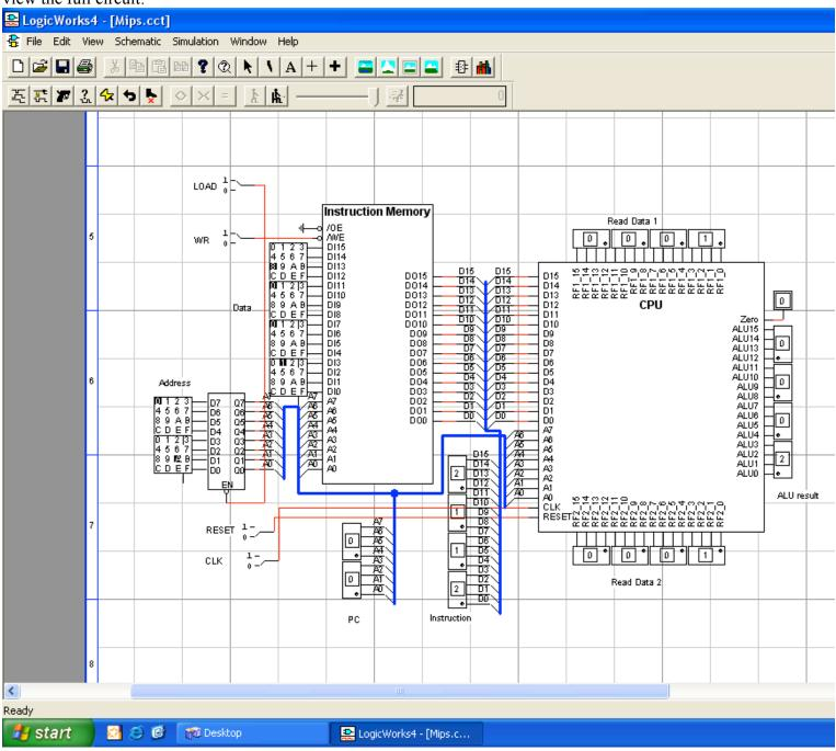
The CPU has been abstracted to a black box, and is connected to the Instruction Memory, where programs must be loaded prior to execution by the CPU. You may recall from an earlier lab that the **LOAD**, **WR**, **data**, and **address** switches on the left are used to load a program into Instruction Memory.
