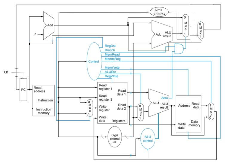
As you have learned in lecture, this machine executes one instruction per clock cycle. The clock cycle must be long enough for the instruction with the longest path (*critical path*), which is the **Iw**. Since many of the instructions executed in a typical program have a shorter path than the **Iw**, the single-cycle datapath is inefficient (it wastes time during the shorter instructions).
