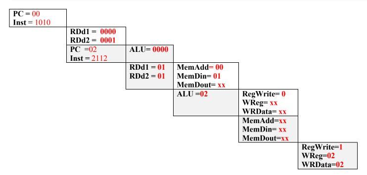
Does it matter what the values are in the **Memory** stage for this instruction? How about the **Writeback** stage? The memory stage does not matter, because it is not a memory access instruction. The writeback stage does matter, because a value is being written back to register 2 as a result of the add.
