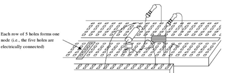
All holes in a row internally connected (use to tie one point to another in the circuit)
