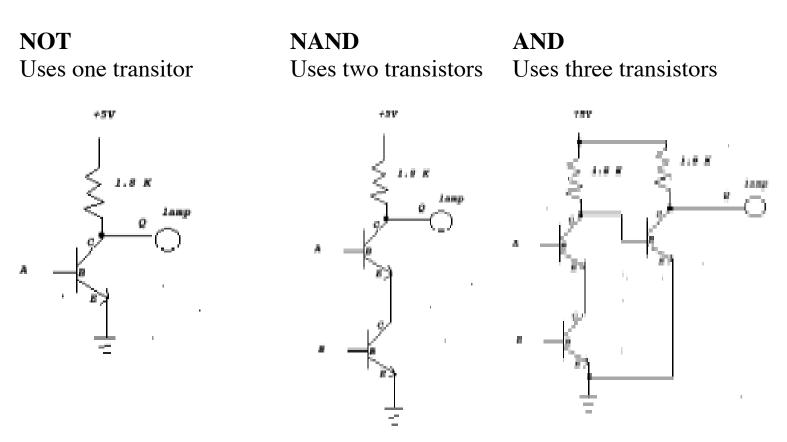
**Voltage levels** can be interpreted as 1s and 0s: all possible inputs and outputs of a circuit can be described using the binary number system.
