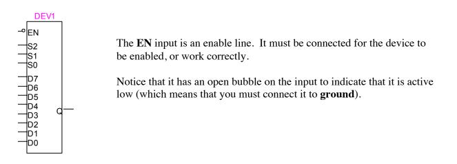
Connect D0 – D8 to **binary switches**. Use a **binary probe** to display your output.
