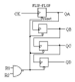
QA serves as the clock to QB. So, QB only changes when QA falls from 1 to 0 (on the negative edge). QB therefore only changes half as frequently as QA.
