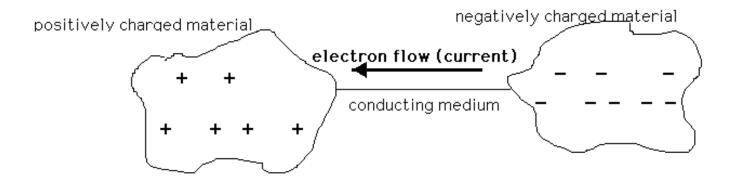
Rate at which electrons flow through = current (A).
