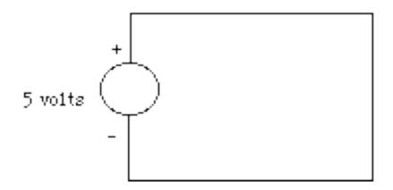
Infinite current swiftly results in the destruction of the circuit!
