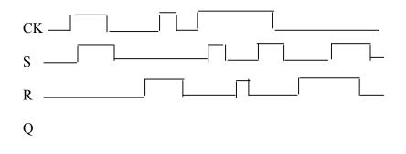
4. Assume you have a clocked SR **flip-flop**, that is activated on the positive edge of the clock. Draw Q given the same CK, S, and R:
