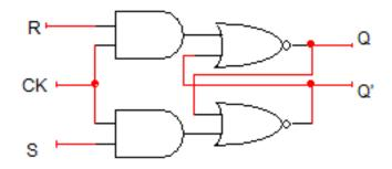
Output Q can change in response to S and R whenever the CK input is asserted.
