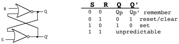
What does **unpredictable** mean? Notice in a NOR gate, if either input = 1 to a gate, its output = 0 (1 is a deterministic input):
